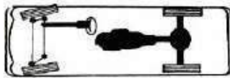
Fig. Centre engine drive.
