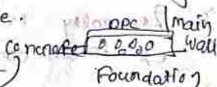
Masonry is computed in cum (length  $\times$  breadth  $\times$  height). Foundation and plinth masonry is taken under one item, and masonry in super structure is taken under a separate item.
