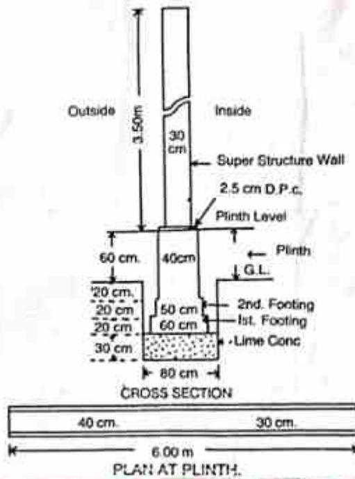
**DETAILS OF MEASUREMENT AND CALCULATION OF QUANTITIES**
