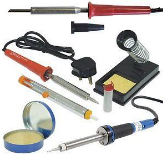
Figure 6.2 soldering irons with solder wire and flux stock
