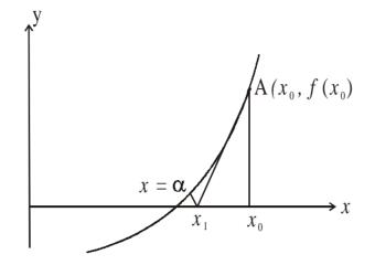
In this method, instead of taking two initial rough approximations to the root  $x = \alpha$  as in the previous two methods, a single rough approximation  $x_0$  to the root is taken. Then we use the following formula, known as Newton-Raphson formula or Newton iteration formula, to get the successive approximations.
